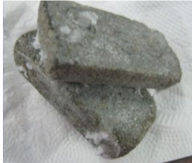
Precipitation on concrete specimen
